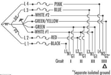
System is rated for connection to a ground 120/240V, 1-PH 60-hz, 20 amp multi-wire branch circuit
